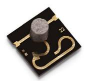
Our new SMT microstrip solution is true surface mount with no need of any additional biased steel plate for installation. The new solution covers K, Ku and Ka bands, with up to 20dB isolation, 1.0dB insertion loss. Custom design microstrip isolators /circulator is available from 5Ghz to 40Ghz. JQL's SMT microstrip series are the smallest and lightest in the industry. As part of our customer's 5G solution, our isolator/circulator has been used in the MIMO antenna.
