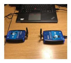
8. The SDR configuration uses ADALM-PLUTO radios (left). Also shown is a corresponding confusion matrix (right). (© 1984–2019 The MathWorks, Inc.)
